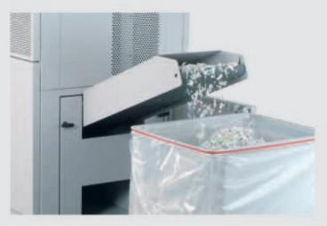
The modular conveyor belt system (available at an extra cost) locks into the shred exit area.
