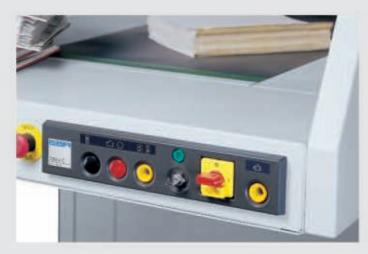
The control panel is conveniently integrated into the feeding table for easy operation.
