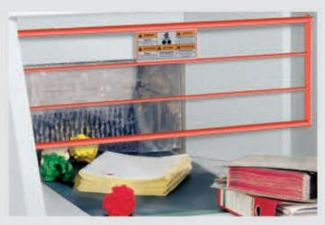
The hinged safety guard in the feeding area is electronically secured. The shredder stops when the guard is opened.
